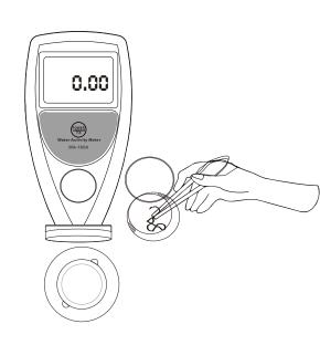
3. Open the container dish and put the test sample into the container dish
